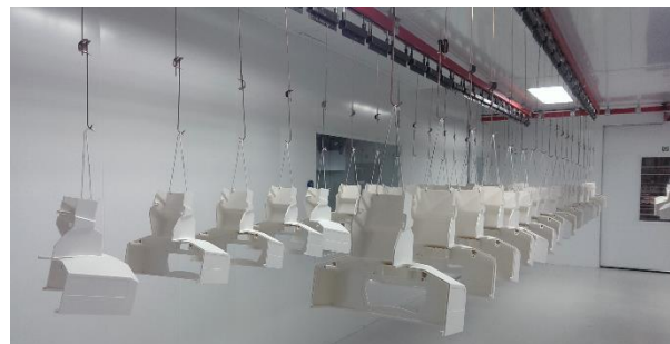
Liquid spray coating in a professional coating cabin.
