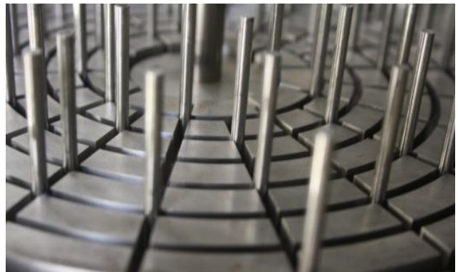
Detail of a mould with long, thin ejectors.
