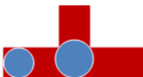
Rib as thick as wall. The circles inside show the difference in the amount of material used.
