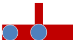
Rib thickness approx. 50% of the wall. The material distribution is far better and yields vastly improved shrinkage distribution.
