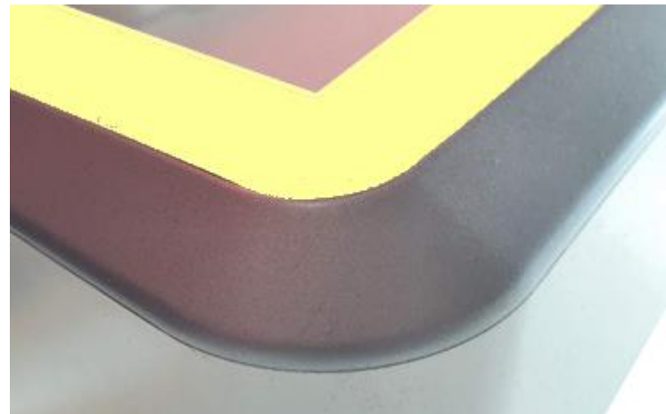
The edge of this white product is painted with a metallic-coloured paint. Pre-punched stencils are used to mask the plastic properly.
