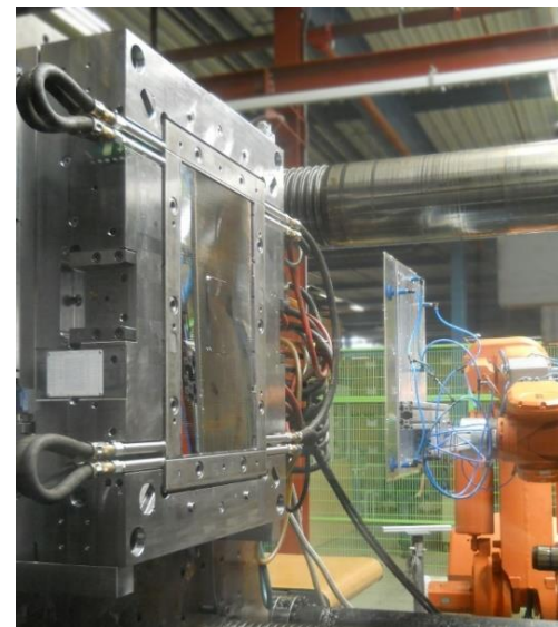
Removal of the first Fresnel lenses from the mould
