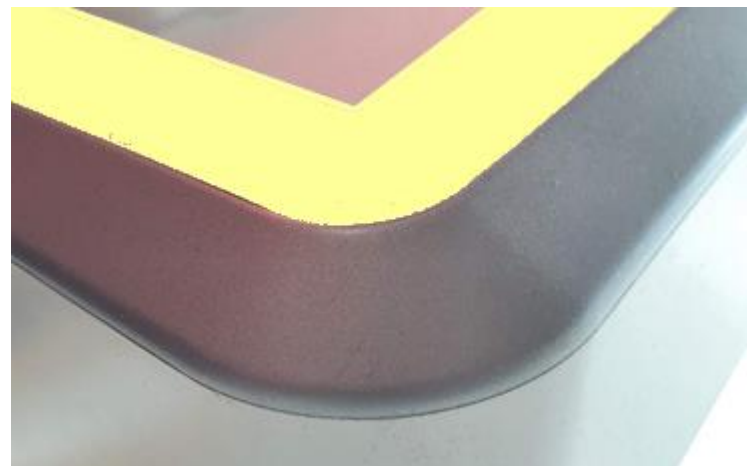
The edge of this white product is painted with a metallic-coloured paint. Pre-punched stencils are used to mask the plastic properly.
